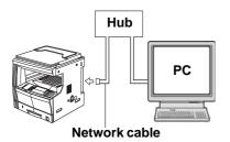
Connecting the scanner to your computer network with a network cable (100BASE-TX and 10BASE-T) page 2-2
