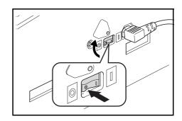
**Caution** ALWAYS turn the main switch to the scanner OFF BEFORE connecting the network cable.
